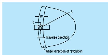
Stock removal is the cutting of the workpiece by the diamonds at the contact surface.
