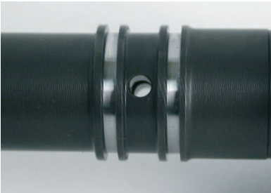
PCBN tool Grooving (finish)
